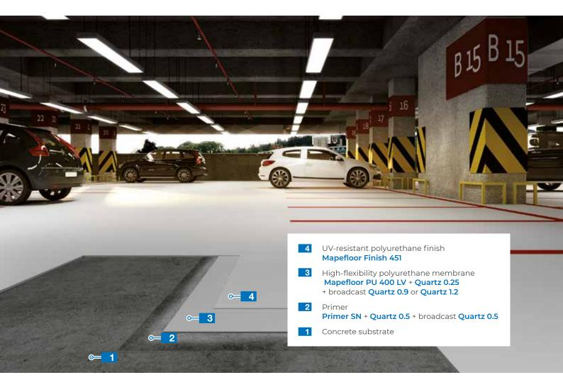
Flexible, slip-resistant, multi-layered, coloured coating system with crack-bridging capacity at temperatures down to -20°C. Suitable for creating strong, impermeable and waterproofing\* coatings with high chemical resistance on internal surfaces, including those subjected to variations in temperature.
