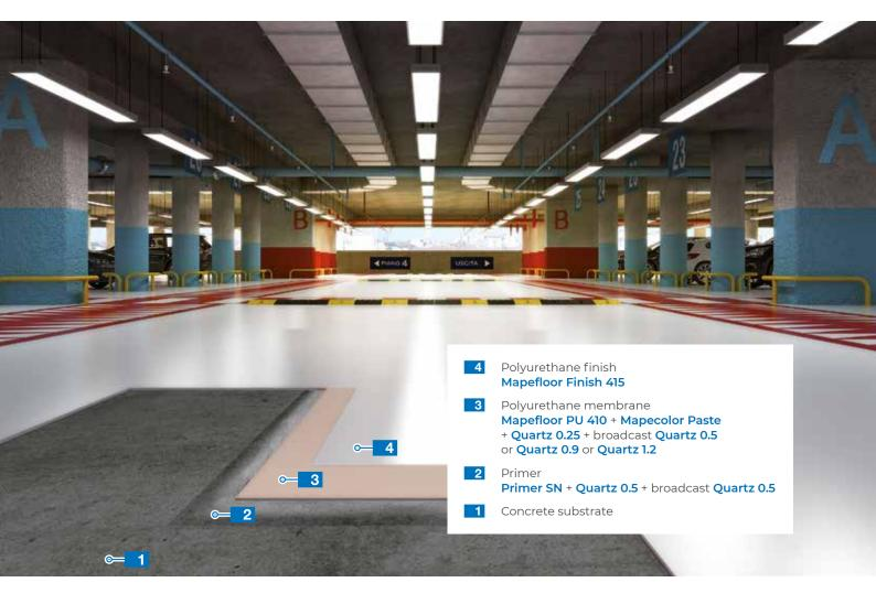
Flexible, slip-resistant, multi-layered, coloured coating system. Suitable for creating strong, waterproofing\* coatings with high chemical resistance on internal surfaces, including those subjected to moderate variations in temperature.
