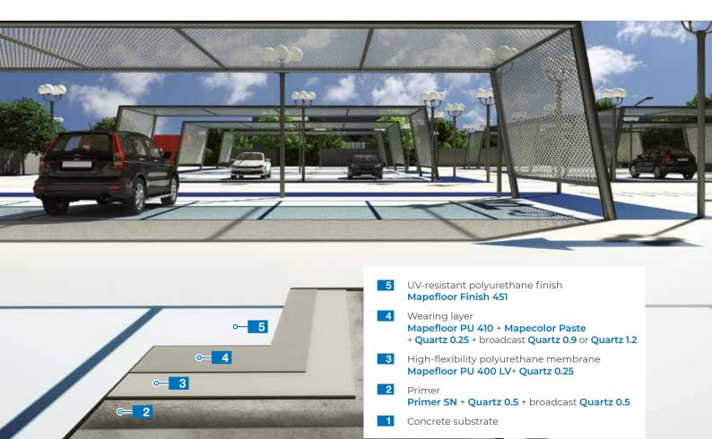
Highly flexible, slip-resistant, multi-layered, coloured coating system with crack-bridging capacity down to -20°C. Suitable for creating strong, waterproofing\* coatings with high chemical resistance on both internal and external surfaces.
